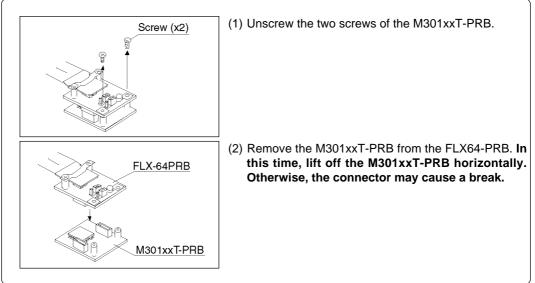
Figure 3.10 Removing pod probe M301xxT-PRB
